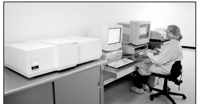
Spectrophotometry used to measure the spectral performance of thin-film coating designs
