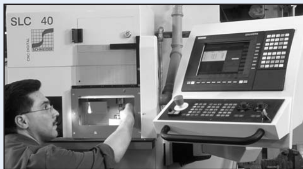
Automated CNC equipment for edging and beveling
