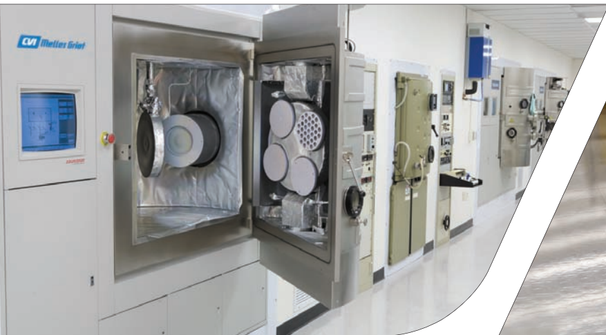
Dedicated state-of-the-art ion-assisted beam sputtering for high efficiency, high reliability lasers with controlled and repeatable spectral output.
