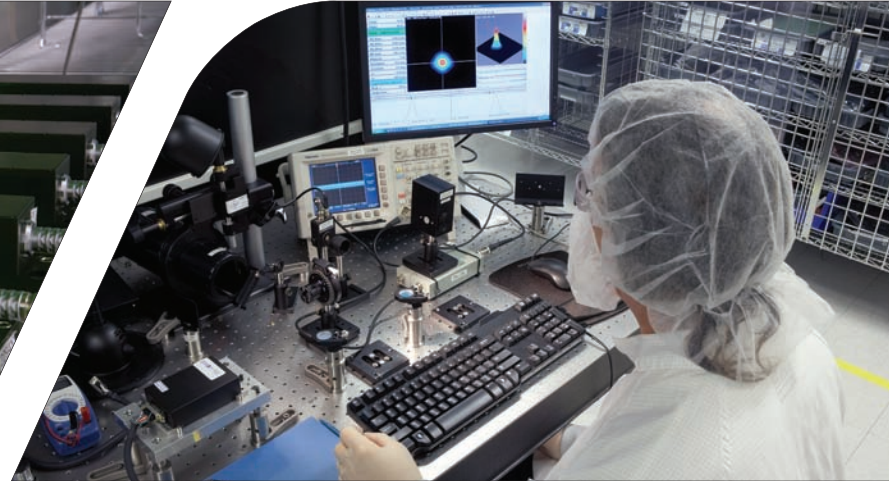
Automatic verification testing of lasers for power stability, optical noise and beam output characteristics.
