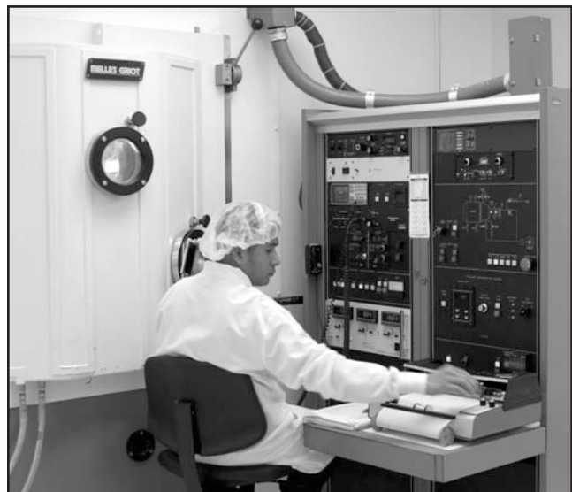
CVI Melles Griot deposition system
